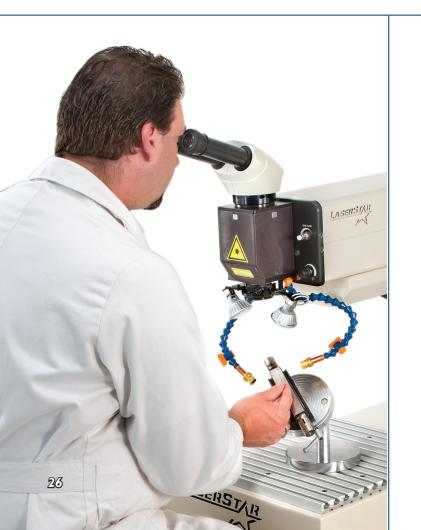
LaserStar welding systems are ideal for a wide range of large plastic injection mold, tool & die maintenance and repair applications.
